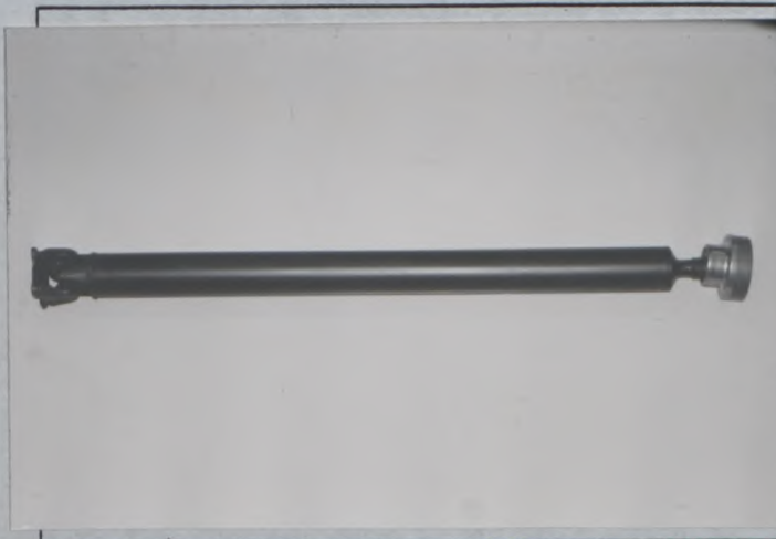
PHOTO Z1 REINFORCED PROPELLER SHAFT
