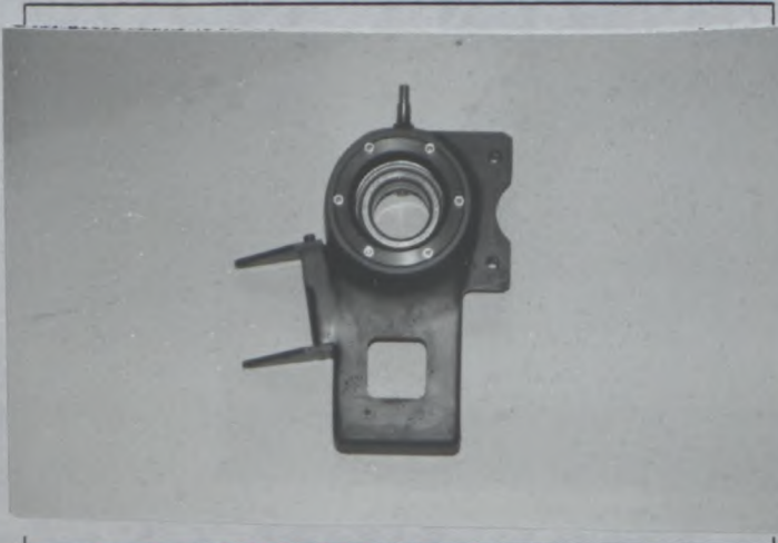
PHOTO T3 REINFORCED KNUCKLE
