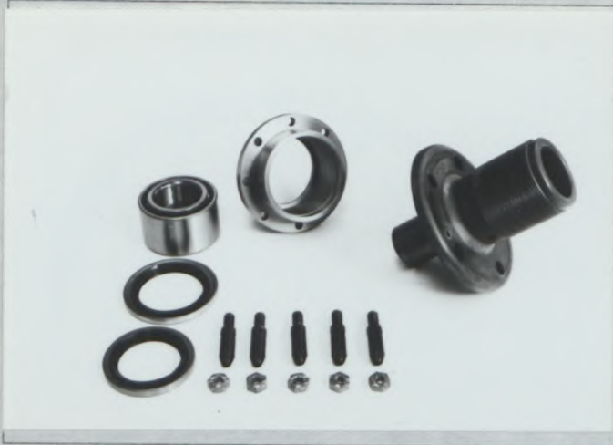
PHOTO U2 CENTRAL WHEEL BOLTING SYSTEM
