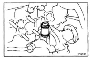
(d) Remove the No.1 water bypass pipe and 2 O-rings.
