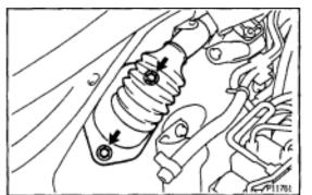
(c) Remove the 2 bolts holding the engine wire retainer to the cowl panel.
