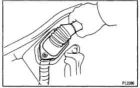
(h) Pull out the engine wire from the cabin.
