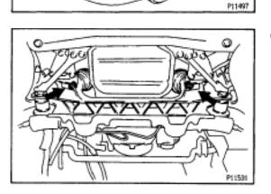
(b) Remove the 2 nuts holding the engine front mounting insulators to the front suspension crossmember.
