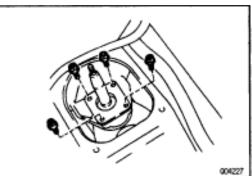
(e) Remove the 4 bolts holding the shift lever to the shift lever retainer.
