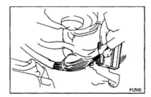
Disconnect the connector from the connector cassette. (g)
