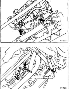
**16. DISCONNECT PS PRESSURE TUBE FROM ENGINE** Remove the 2 clamp bolts, and disconnect the pressure tube.
