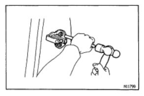
(d) Using a brass bar and hammer, tap the striker to adjust it. **CAUTION: Do not tap the striker too hard.**
