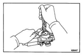
(b) Pull out the drum while detaching the cable guide out from the motor.
