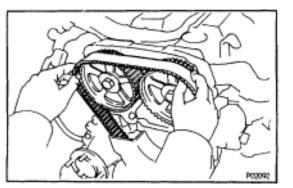
(a) Alternately loosen the 2 bolts, and remove them, the tensioner and dust boot.
