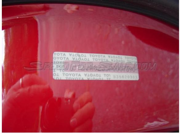
10. **Rear passenger's quarter panel:** located on the side of the passenger's door jamb.
