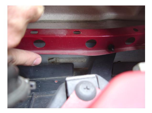
5. **Firewall Stamp:** This is NOT a tag/sticker, it is etched / stamped into the metal. It is located underhood on the passenger firewall, just beside the black 'DIAGNOSTICS' box on the passenger side firewall and directly behind the turbocharger(s). It should start out with JZA80 – followed by the last few numbers of the VIN number.
