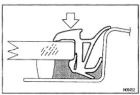
3. **INSTALL WINDSHIELD MOULDING** Place the moulding onto the body and tap it by hand.
