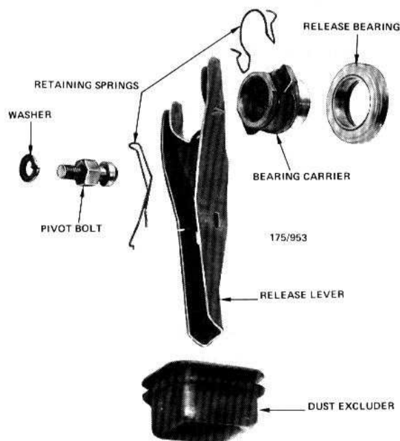
Dismantled view of clutch release components.
