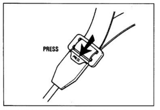
To release the belt; press the release button (marked "PRESS") located on he front face of the buckle and the tongue will be released.
