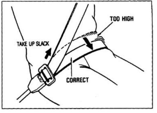
The lap belt should fit snugly and as low as possible on your hips, not on your waist. Adjust it to a snug fit by pulling the shoulder portion upward through the latch plate. Failure to do so could increase the chance of injury due to sliding under the lap belt during an accident. For your safety, do not place the shoulder belt under your arm.
