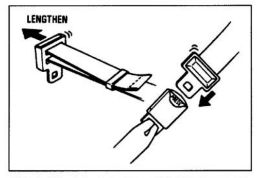
If the belt length has to be increased, hold the tongue at a right angle to the belt and pull on it.
