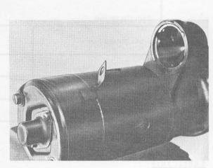
Bolt cap of commutator bearing in place. Connect the solenoid plunger and bolt solenoid switch to drive housing. Connect terminal of winding to solenoid
