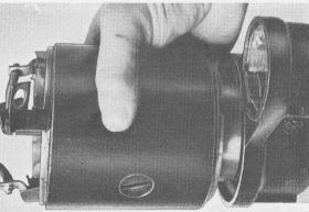
Place armature in a vise. Press actuating sleeve against the overrunning clutch and take it off the armature shaft, watching the locking balls.
