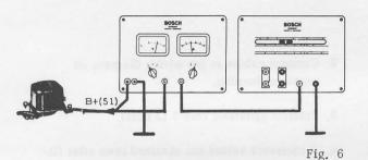
With the sliding resistance increase loading up to maximum capacity of generator. With any further increase of load the voltage must drop.
