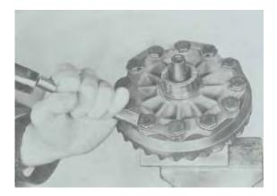
When replacing outer races of side bearings, heat transmission housing or the cover, to approx. 120° C (248° F) and install outer races with an appropriate tool.
