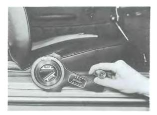
To achieve the specified values in the rear wheel camber adjustment, it is of importance that the adjusted angle of the radius arm is same on both sides of the car. If the radius arm has been adjusted on one side, the other side should be checked as well and its adjustment corrected when necessary.
