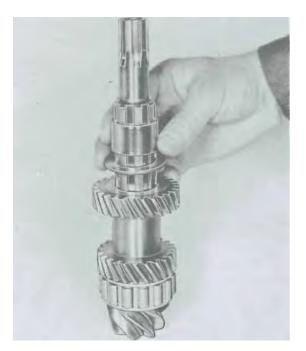
7. Install needle bearing cage, Gear II of 3rd speed, and spider.
