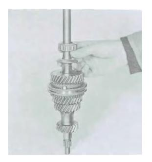
Press roller bearing onto shaft using hydraulic press VW 400F with VW 401, VW 409, and pipe piece 1 (20x3. 5 mm, 25 mm long).
