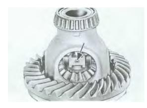
2. Remove the shaft with a punch and take out anchor piece.
