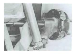
8. Drive the rear hub out with special tool P 297.
