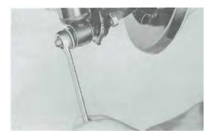
15. Remove self-locking nut of the control arm mounting bolt and drive the bolt out with the aid of a punch. At that time move the control arm slightly so that the bolt can clear the transmission housing. If necessary, slightly loosen the transmission carrier retaining bolts.
