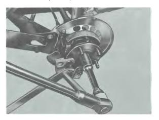
at the joint flange. Separate the halfshaft from the joint flange using a flat chisel along the flange gasket, and take off the halfshaft.
