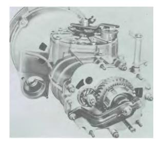
7. Insert dial gauge into holder. Tighten holder look screw and holder retaining bolt (screwed into differential shaft) so that the gauge sensor pin comes into contact with the base of the clutch conduit bracket.
