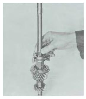
Fig. 73 Caution: Used needle bearing cages have to be reinstalled with the same gear.
