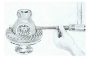
3. Turn the pinions so that the small pinions can be taken out through the side openings in the differential housing. Remove the large pinions together with the threaded lock pieces. Do not interchange the shims or spacers. Attach tags to prevent mixing up right side with left side and vice-versa.
