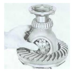
7. Install the pinion shaft while holding the anchor piece thereby preventing the anchor piece from binding on the shaft during installation.
