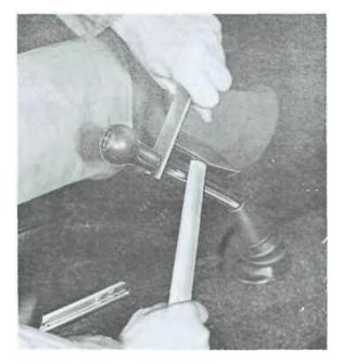
2. Pull internal locking ring out of the knob with a suitable hook.
