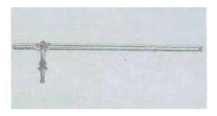
23. Shift into neutral, guide inner shift rod into proper position at selector shaft tabs and into the rear rod bore.
