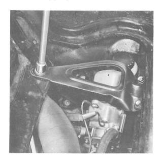
4. Unlock and remove steering coupling retaining bolts.
