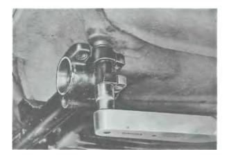
3. Install the crossmember brace without binding forces. Torque hex nuts to 6, 5 mkp (47 lb/ft), and hex bolts to 4,7 mkp (34 lb/ft).
