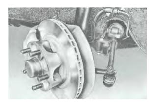
3. Remove ball joint retaining bolt (M 10 x 30) from strut and pull ball joint out of the strut by pushing the suspension control arm downward.
