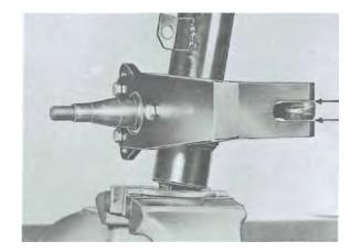
b. The larger diameter of the hole in the steering arm for the track rod joint should not lie outside the test hole in special tool P 284b. (Visual check.)
