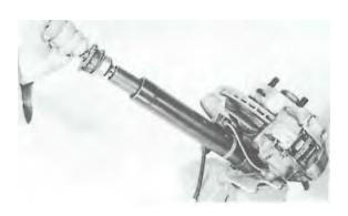
6. Drain the hydraulic fluid from the strut casing and install the new insert.
