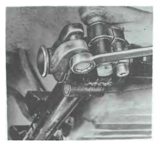
2. Turn the torsion bar adjusting screw back.
