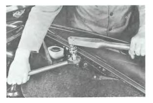
Mount the Shockabsorber strut in a vise equipped with jaw caps. Remove cover tube and take rubber buffer out. Remove insert retaining nut and take out the old insert components.
