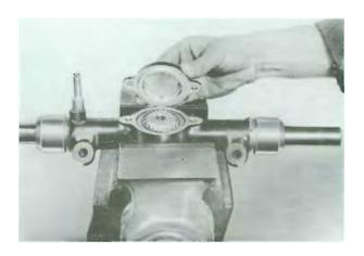
5. Using puller P 293, remove flange from pinion; exercise care as not damage the pinion threads.
