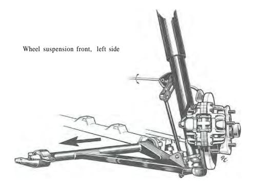
Front wheel springing is effected through an adjustable, longitudinal torsion bar at each wheel. Complementing the springing is a progressively-acting rubber buffer installed in each of the two double-action hydraulic shock absorber struts.
