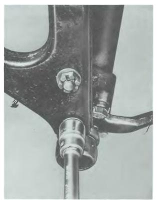
12. Unlock and unscrew hex nut at top of Shockabsorber strut, remove strut.
