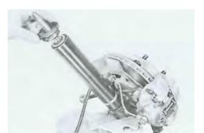
7. Tighten insert retaining nuts:
