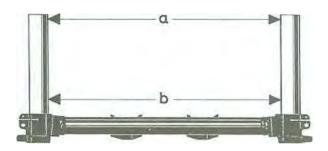
3. Place the reinforcing crossmember onto a flat surface (straightening plate). With one alignment measuring tube laving perfectly flat, check for twist at the other tube with the aid of a feeler gauge. Maximum permissible difference between the flat surface and either end of the tube is 2 mm. Greater deviations necessitate replacement of the reinforcing crossmember.
