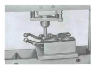
6. Drive distance ring off wheel spindle striking with drift punch at different place.
