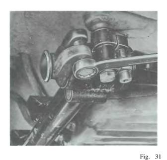
4. Remove retaining bolts from control arm bushing bracket, remove bracket and bracket cap.
