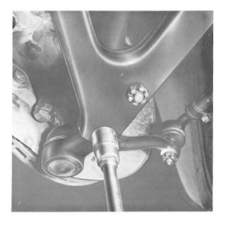
Remove retaining bolts from control arm rubber mount cover bracket and remove bracket.
