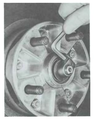
4. Loosen Allen bolt in wheel bearing clamping nut, unscrew nut and withdraw bearing washer.
