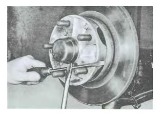
9. Unlock and remove brake carrier retaining bolts, withdraw carrier.
