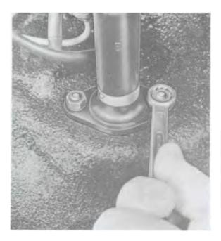
3. Provide a clearance of approx. 1 mm (. 04") between piston rod and piston in master cylinder. (Loosen lock nut on piston rod and turn rod as appropriate).
