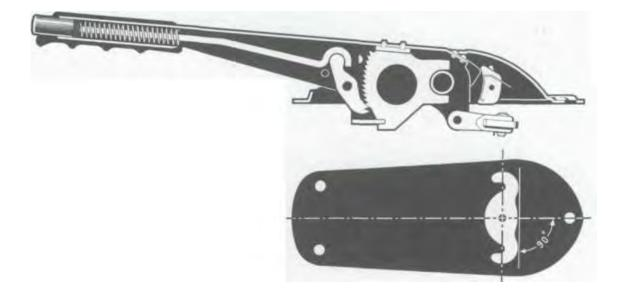
Cross-section of Handbrake Lever with Cable Equalizer Fig. 39
