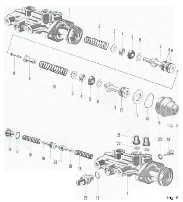
Exploded View of Tandem Brake Master Cylinder (for USA)
