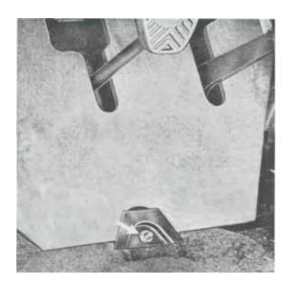
Detach brake lines from brake master cylinder. (In USA-type vehicles also detach wires from circuit failure sender.)
