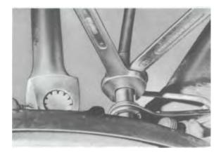
4. Insert screwdriver into opening in drum of rear brake disc assembly and turn handbrake adjusting sprocket until tight, that is, so that the brake disc can no longer be turned by hand.
