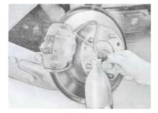
3. Repeatedly depress the brake pedal in quick succession (pumping) until a slight pressure becomes evident, then hold the pedal under pressure while opening the bleeder valve by about 1/2 to 3/4 turn, and quickly depress the pedal to floor. Before releasing the pedal, always close the bleeder valve first, then allow the pedal to return slowly.
