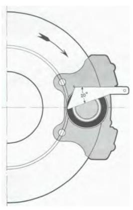
With caliper installed, the piston aligner ( P 84) must always rest against the upper edge of the brake pad slot.
