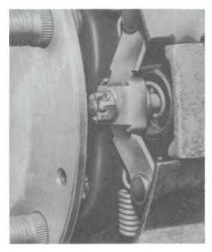
10. Raise upper brake shoe with a screwdriver, withdraw adjusting assembly, and unhook spring.
